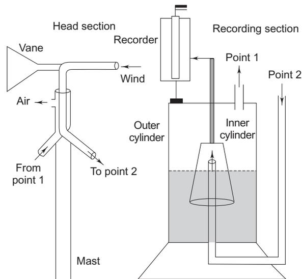
**Fig. 2.2** The pressure tube anemometer
