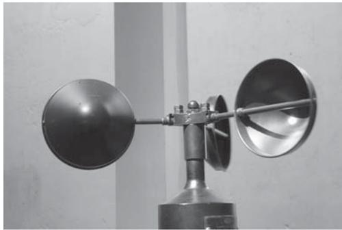
**Fig. 2.1** The Robinson cup anemometer
