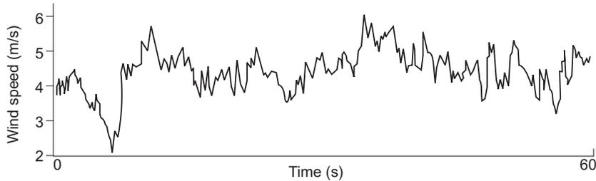
**Fig. 2.3** Typical anemometer recording of wind speed versus time
