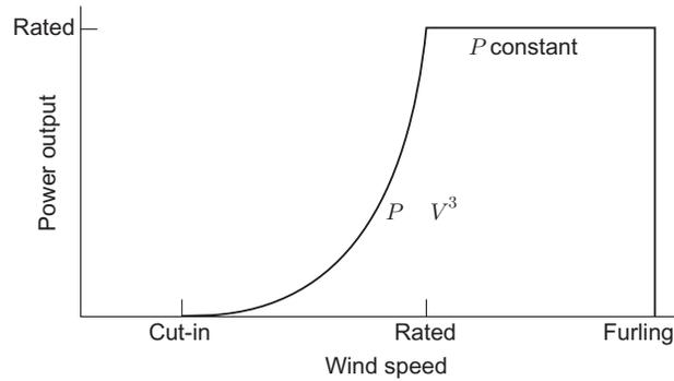
**Fig. 2.8** Typical power versus wind speed characteristics of constant-speed wind machines
