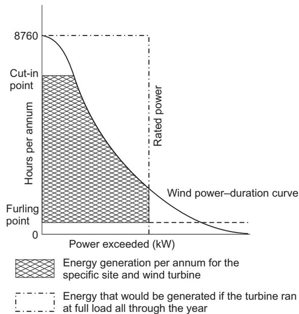
**Fig. 2.9** The output power-duration characteristics of a wind generator at a given site
