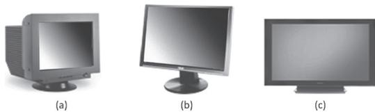
**Figure 1.34** (a) CRT monitor (b) LCD monitor (c) Plasma monitor
