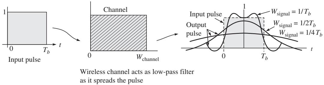
**Fig. 1.4** Response of an ideal pulse transmitted through a channel according to the bit rate over a fixed channel bandwidth
