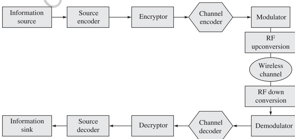
Fig. 1.3 Basic model of wireless digital communication link
