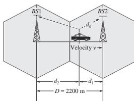
Fig. 2.13 Two base station scenario for handoff calculations
