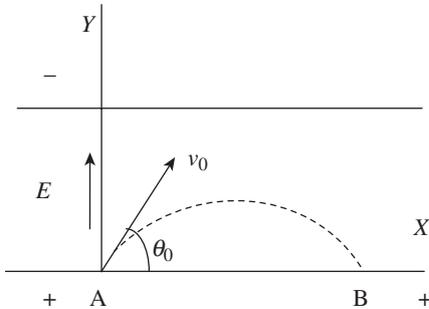
**Fig. SN.1** Parabolic path of an electron in uniform electric field
