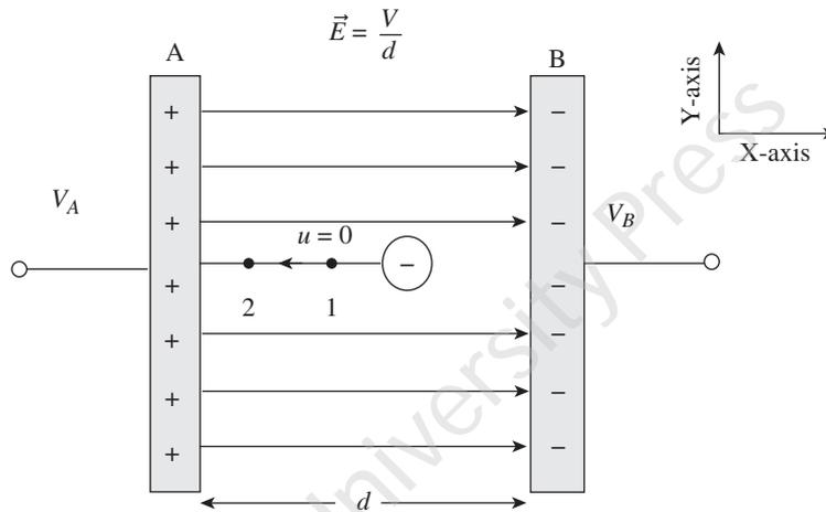
Fig. 1.13 Motion of electron in uniform longitudinal electric field
