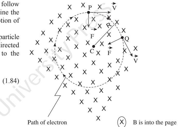
**Fig. 1.18** Force exerted by a uniform magnetic field on a moving charged particle (in this case, an electron) produces a circular path
