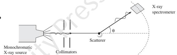
Fig. 3.2 Experimental arrangement of Compton effect
