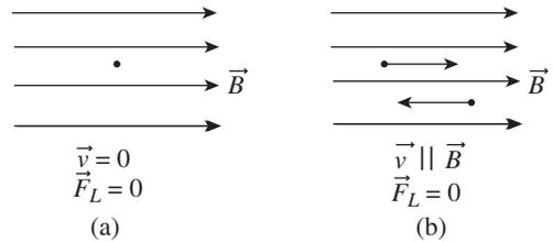
**Fig. 1.17** Electron in a uniform magnetic field. (a) When a charged particle (positive or negative) is at rest (b) When a charged particle (positive or negative) is moving parallel or antiparallel
