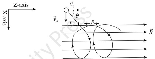
**Fig. 1.19** An electron entering in a magnetic field at an angle  $\theta$  spirals about the field lines
