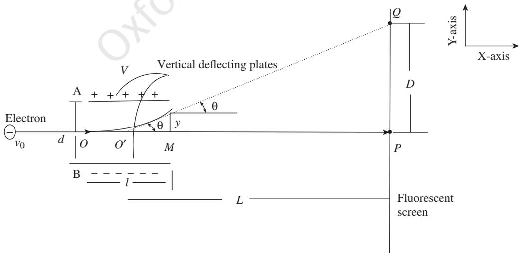
Fig. 1.14 Electron motion in transverse uniform electric field
