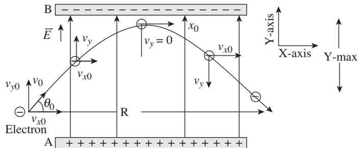
**Fig. 1.15** Projectile motion of an electron in a uniform electric field.
