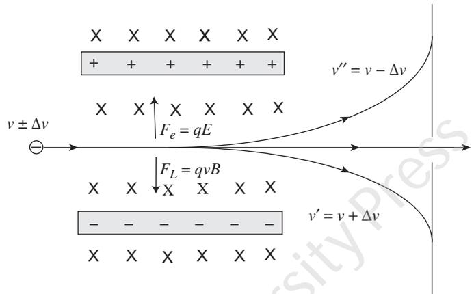
**Fig. 1.20** Crossed field configuration as a velocity filter/selector
