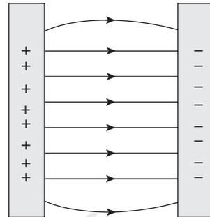
**Fig. 1.5** Uniform electric field produced by a parallel plate capacitor. Field is non-uniform at the edges
