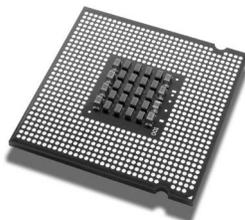
Physically, it is an integrated circuit (IC) silicon chip, mounted on a small square plastic slab, surrounded by metal pins. In the world of personal computers, the term microprocessor and CPU are used interchangeably. It is more accurate to describe it as a CPU on a chip because it contains the circuitry that performs processing.
