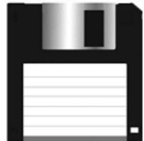
and can store 1.44 MB of data. Earlier PCs sometimes used 5¼ inch disks. The disks store information and can be used to exchange information between computers. The floppy disk drive stores data on and retrieves it from the magnetic material of the disk, which is in the form of a disk. It has two motors one that rotates the disk media and the other that moves two read-write heads, each on either surface of the disk, forward floppy disk drive or backward.
