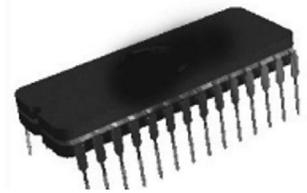
EPROMs (Erasable Programmable Read Only Memories). In the EPROM data can be written electrically. The write operation, however, is not simple. It requires the storage cells to be erased by exposing the chip to ultraviolet light, thus bringing each cell to the same initial state. This process of erasing is time consuming. Once all the cells have been brought to the same initial state, the write operation on the EPROM can be performed electrically.
