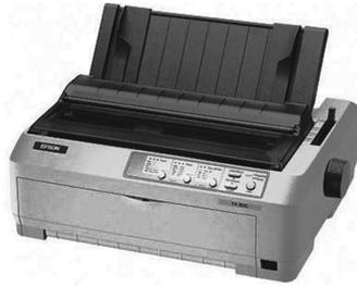
a text or an image. An *impact printer* is one where the print head will be in physical contact with the paper. In a *non-impact printer*, on the other hand, the print head will have no physical contact with the paper. The dot matrix printer is considered as an impact printer and laser printer is considered as non-impact printer.
