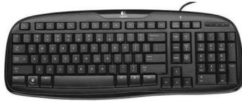
Each key holds a position with respect to a row and column. When a key is pressed, the key switch in that position closes a circuit, sending a signal to the circuit board inside the keyboard. The keyboard controller uses the x and y coordinates of the matrix position to determine which key was pressed, thereby determining the code transmitted to the computer by the keyboard.
