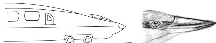
**Figure 1.1** The nose of the re-designed Shinkansen, shaped like a kingfisher's beak
